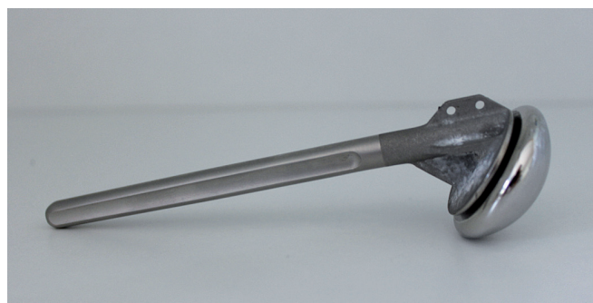
Figure 4. A modular stemmed hemiarthroplasty with the head connected to the stem by a taper locking system with the possibility of different head-stem combinations depending on the size of humerus.
