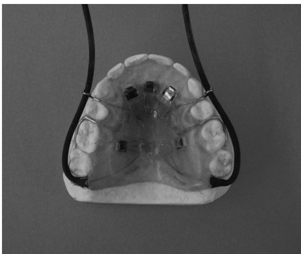
Figure 5. Photograph of prototype pressure-sensing palate, with five embedded pressure sensors (three in anterior region and two posterior).
