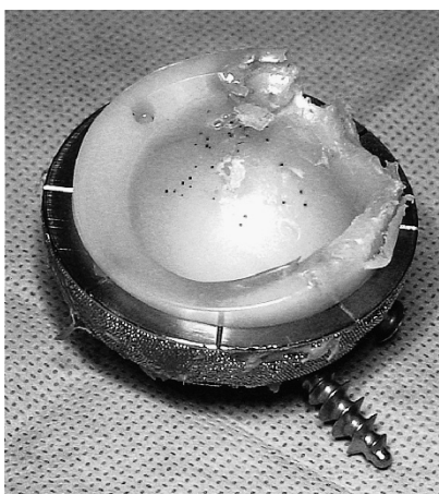
Figure 2. Extensive bead embedding in the polyethylene articular surface of a porous acetabular component of a different design.
