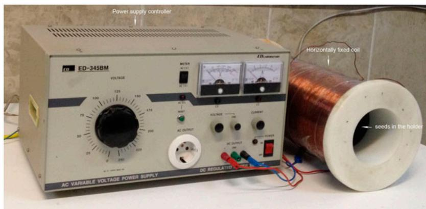
Figure 1. Electromagnetic field generator for seed treatment.
