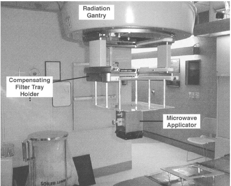
Figure 1. A Clinitherm  $10 \times 10\text{ cm}^2$  applicator mounted to a blocking tray that is mounted to a compensating filter tray via an aluminum frame. The SSD at the bottom of the applicator is 100 cm and 101.5 cm at the patient microwave bolus interface. The compensating filter tray holder is used to attach the applicator to the gantry, to ensure reproducibility, and to eliminate problems with blocking radiation fields.
