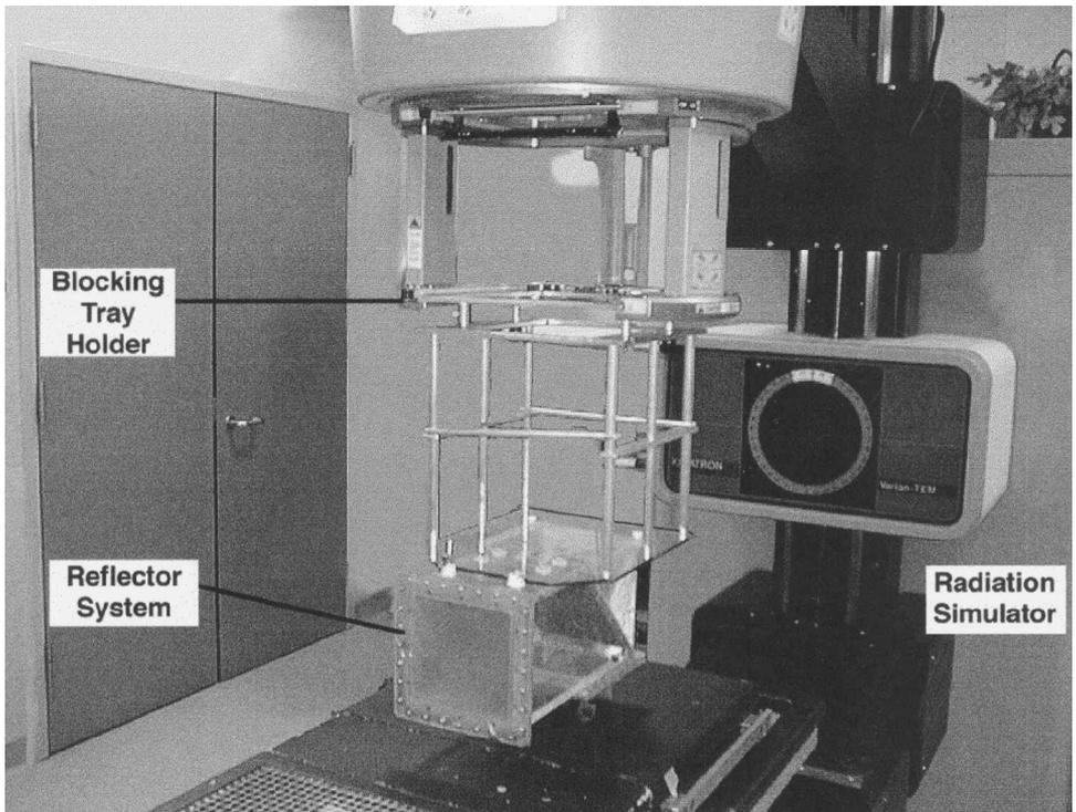
Figure 3. The reflector system mounted to the gantry of the radiation simulator. A special attachment is used to insert the reflector system into the blocking tray of the simulator gantry while maintaining the same distance from the reflector system to the radiation source that is attained in the linear accelerator set-up. This set-up is used to determine the SSD that achieves optimal coupling and to ensure that the ultrasound system can be coupled to the patient effectively.
