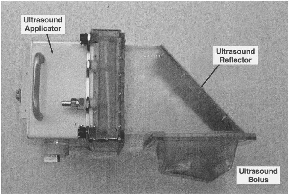
Figure 7. A photograph of the 16-element ultrasound applicator (Sonothem 1000, Labthermics Technologies, Champaign, IL) with a reflector attached to the applicator. The reflector is necessary in some cases when the orthogonal technique is used because of the height mismatch between the position of the patient for radiation therapy and the support system for the Sonothem 1000.
