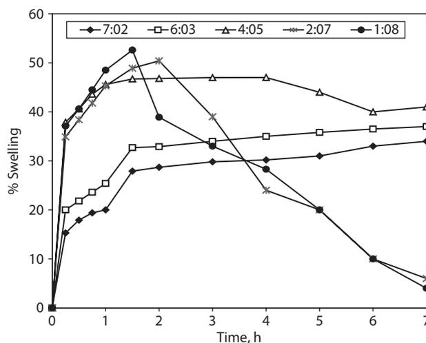
**Figure 5.** Water uptake (swelling %) of compacted matrix-forming components.
