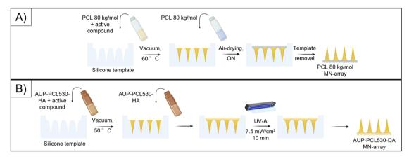
Figure 1. Scheme representing the molding procedure. (a) represents the vacuum molding of the PCL 80 kg/mol-based MN arrays, while (b) shows the vacuum molding procedure for the AUP-PCL530-HA-based MN arrays. The illustration was prepared with Biorender.
