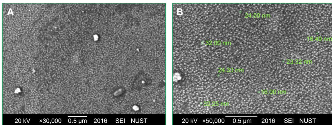
**Figure 4** SEM images of green synthesized CeO<sub>2</sub> NPs. (A) Magnification  $\times 30,000$ ; (B) Magnification  $\times 50,000$ .
