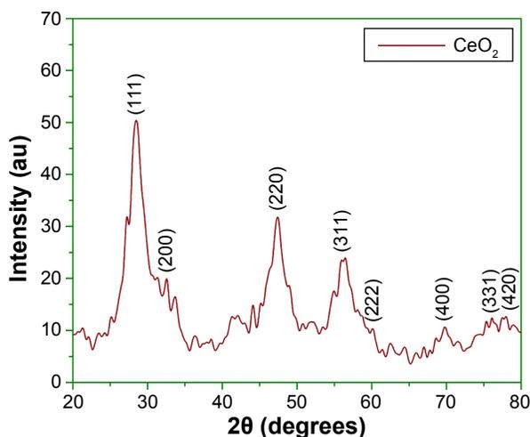
**Figure 6** Typical XRD analysis of CeO<sub>2</sub> NPs at room temperature.
