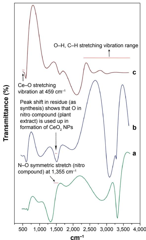
**Figure 7** FTIR spectra of biosynthesized CeO<sub>2</sub> NPs from *Olea europaea* leaf extract.
