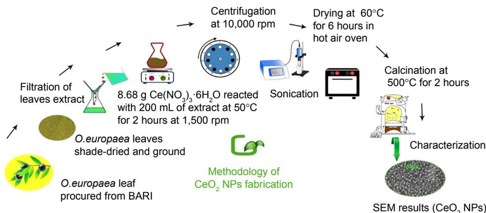
**Figure 1** Schematic diagram of fabrication of CeO<sub>2</sub> NPs using *Olea europaea* leaf extract.
