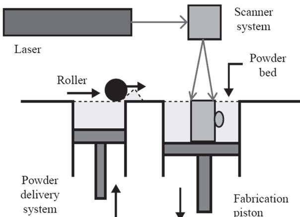
Figure 4. Schematic of the SLS technology. Adapted from reference (48) with permission of Rapid Prototyping Journal, Emerald, Copyright 2009.
