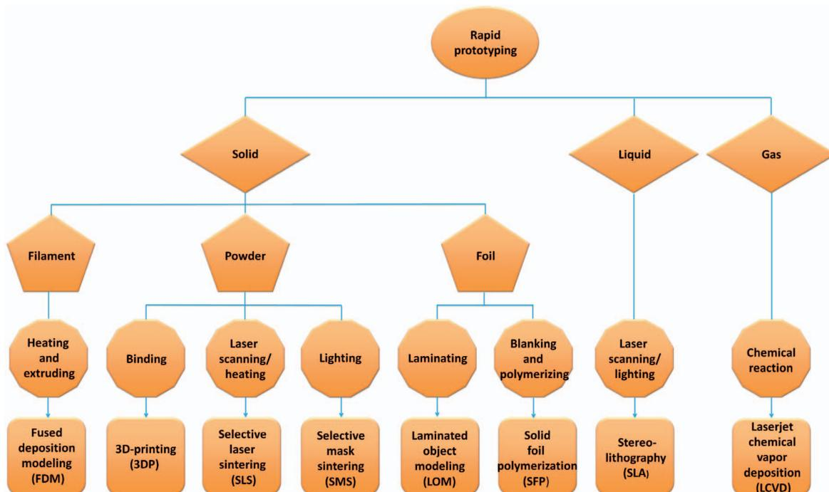
Figure 2. Overview of RP technologies. Adapted from reference (50) with permission of Macromolecular Materials and Engineering, John Wiley and Sons, Copyright 2008.
