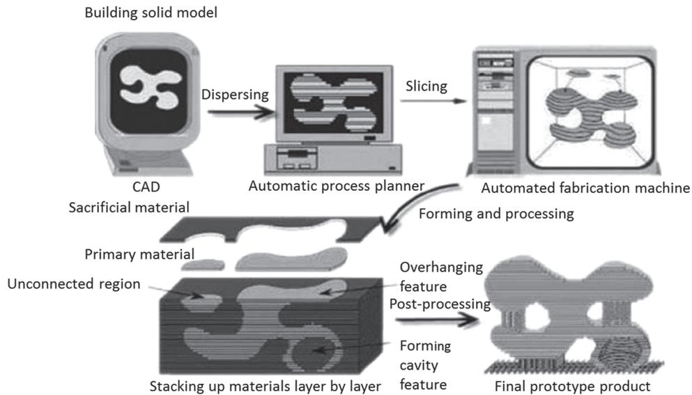
Figure 1. RP process chain showing main process steps. Adapted from reference (48) with permission of Rapid Prototyping Journal, Emerald, Copyright 2009.
