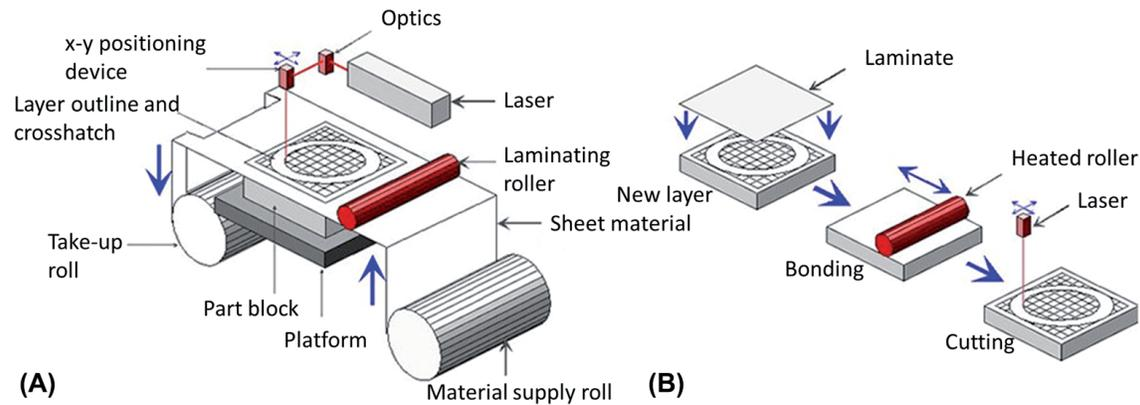
Figure 6. Schematic of the LOM technology. (A) Heating. (B) Bonding. Adapted from reference (72) with permission of Manufacturing Practices, Indian Institute of Technology Delhi, Copyright 2012.
