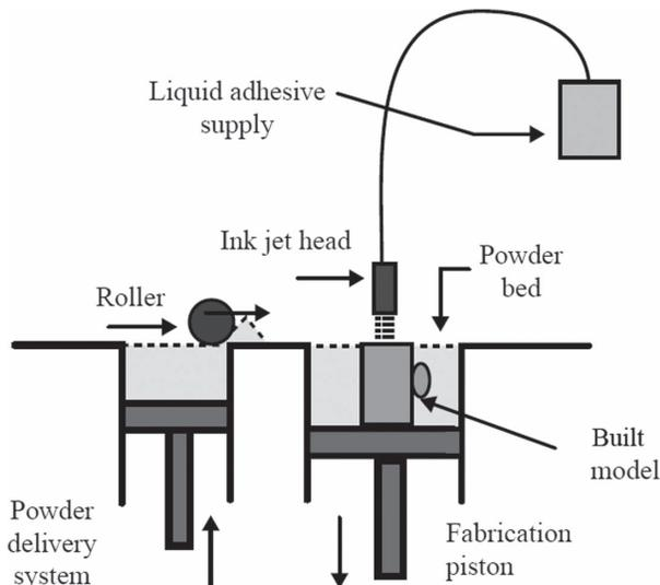
Figure 7. Schematic of the 3DP technology. Adapted from reference (48) with permission of Rapid Prototyping Journal, Emerald, Copyright 2009.
