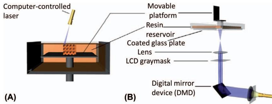
Figure 3. Schematic of two types of SLA setups. (A) A bottom-up system with a scanning laser. (B) A top-down setup with digital light projection (DLP). DLP is a method to illuminate the resin. A 2D pixel pattern is projected onto the coated glass plate with a digital mirror device (DMD), and then a complete resin is cured immediately. Adapted from reference (54) with permission of UTpublications, University of Twente, Copyright 2010.
