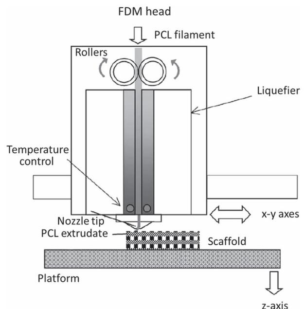
Figure 5. Schematic of the FDM technology. Adapted from reference (70) with permission of Biomaterials, Elsevier, Copyright 2002.
