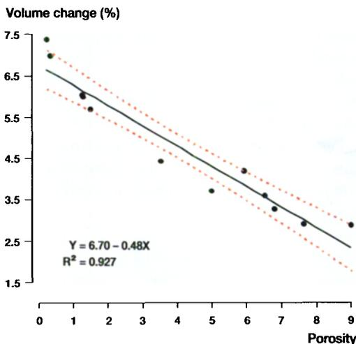
Figure 4. Regression plot of contraction versus porosity (black) + 95% Confidence Interval of line (red).
